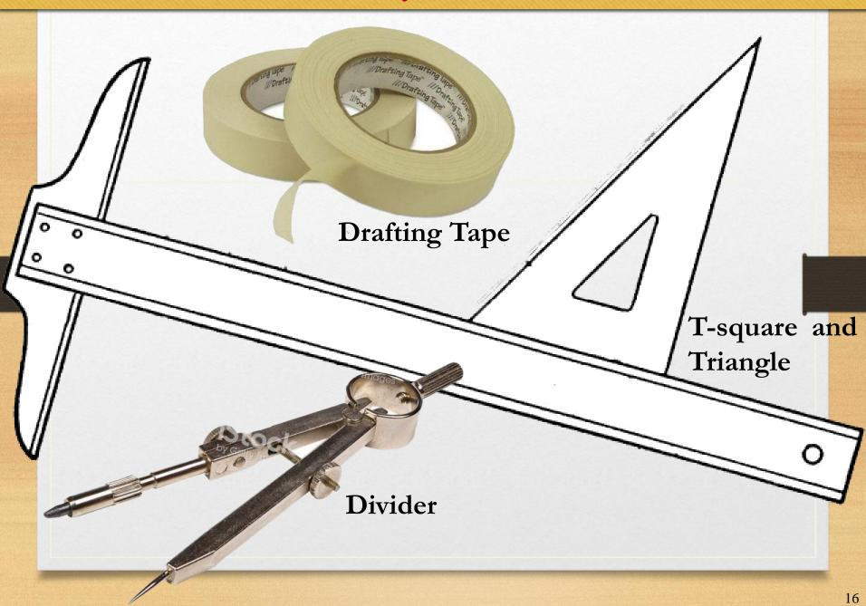
How to Use T-square and Triangles The T extension at the end of the T-square should always remain aligned with the side of the drawing table. This will cause it to remain horizontal. 60° 17
